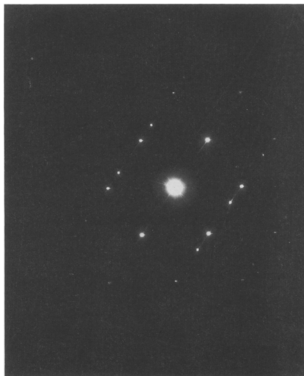
Figure 22 Electron diffraction pattern (SAED) for a single SiC whisker (American Matrix).
