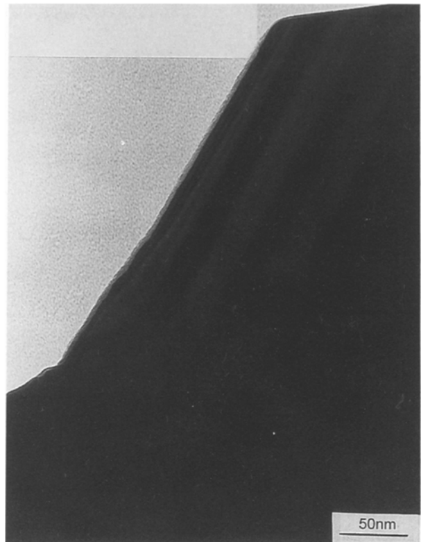
Figure 13 Transmission electron micrograph of American Matrix SiC whiskers possessing a thin coating (3 nm).
