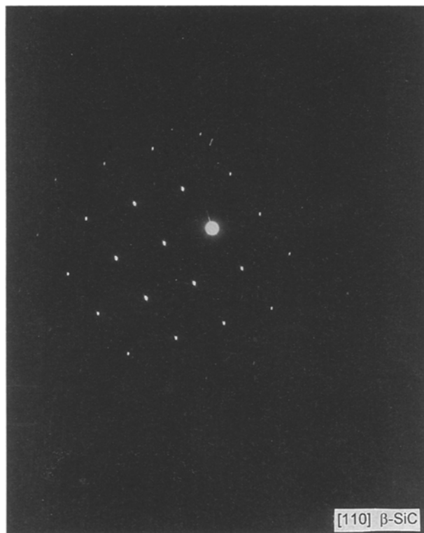
Figure 20 Electron diffraction pattern (SAED) from a single SiC whisker (Tokai).
