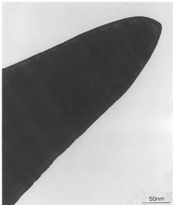
Figure 12 Transmission electron micrograph of tip of Tokai SiC whiskers.
